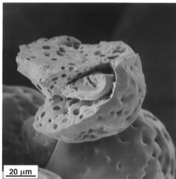
Figure 3. Scanning electron micrograph showing macropores visible on the inside of a broken CLEAR-V bead [ n.b. , the vast majority of beads were intact spheres, but after considerable searching, an accidentally fractured bead was located in the SEM to make this point]. Working magnification: 1000 \times ; accelerating voltage: 10 kV.
